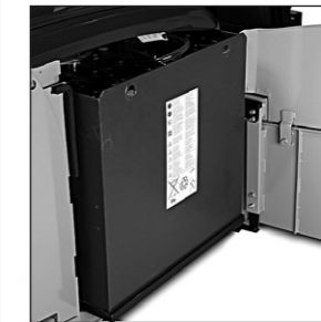
Lateral battery exchange
