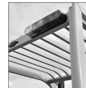
Clear-view overhead guard
